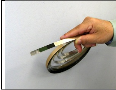
Fig. 3 YBCO superconductor can only be made in long lengths as thin, flat tapes, with critical current density being highly anisotropic for in-plane and out-of-plane magnetic fields.
